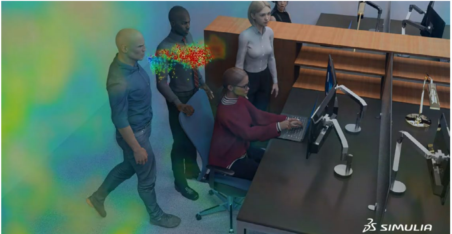
Figure 2: Simulation of a sneeze in an office. The colored air represents airflow from a HVAC system behind the sneezer. © 2020 Dassault Systèmes. All rights reserved. The simulation(s) by Dassault Systèmes and other technical or operational information represented in this article are presented as an illustration and are for informational purposes only. Any use of information presented in or derived from this article is at the viewer's sole risk and Dassault Systèmes disclaims all related liability.
