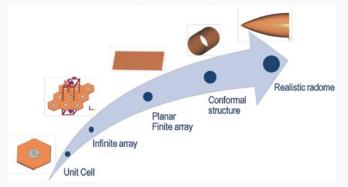
Figure 3. Design and analysis flow for a periodic structure for Radome applications.
