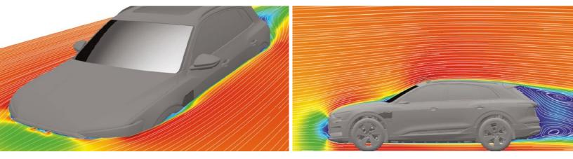
Velocity cut plot post processing in SIMULIA PowerVIZ—Audi Etron aerodynamics
