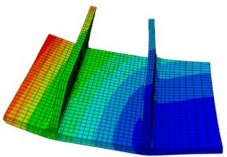
Contour of displacement, magnification 30.
