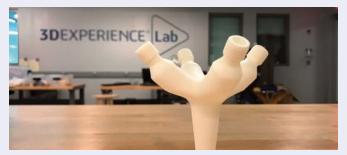
The **3DEXPERIENCE**<sup>®</sup> platform was used to optimize a flow splitter so that it could provide air to multiple patients at one time.
