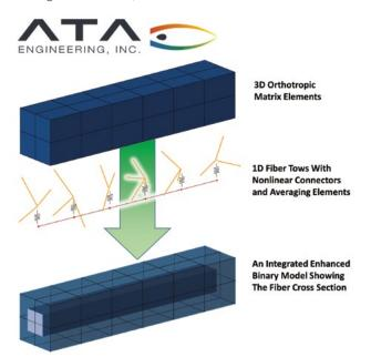
Figure 1. The EBM formulation for composite material architectures.
