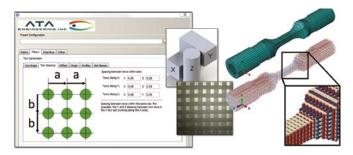
Figure 2. COMPAS automated model generators rapidly create EBMs of arbitrary part geometries.
