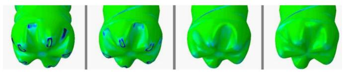
This creasing simulation illustrates how Abaqus makes it easy to test multiple design iterations without the need for expensive prototypes and tooling.
