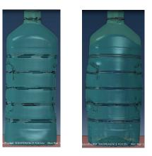
Simulation of container bulging when dropped.
