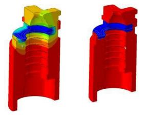
Abaqus can also be used to simulate the manufacturing process. Here, the effects of inadequate mold insulation are easily visualized—on the left is a tool with no insulation, while the right shows one that's been fully insulated.
